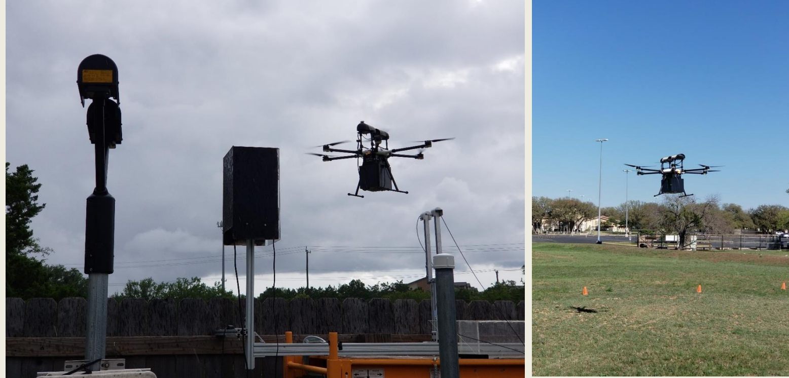
AD for aerial DSD and fall speed measurements.
