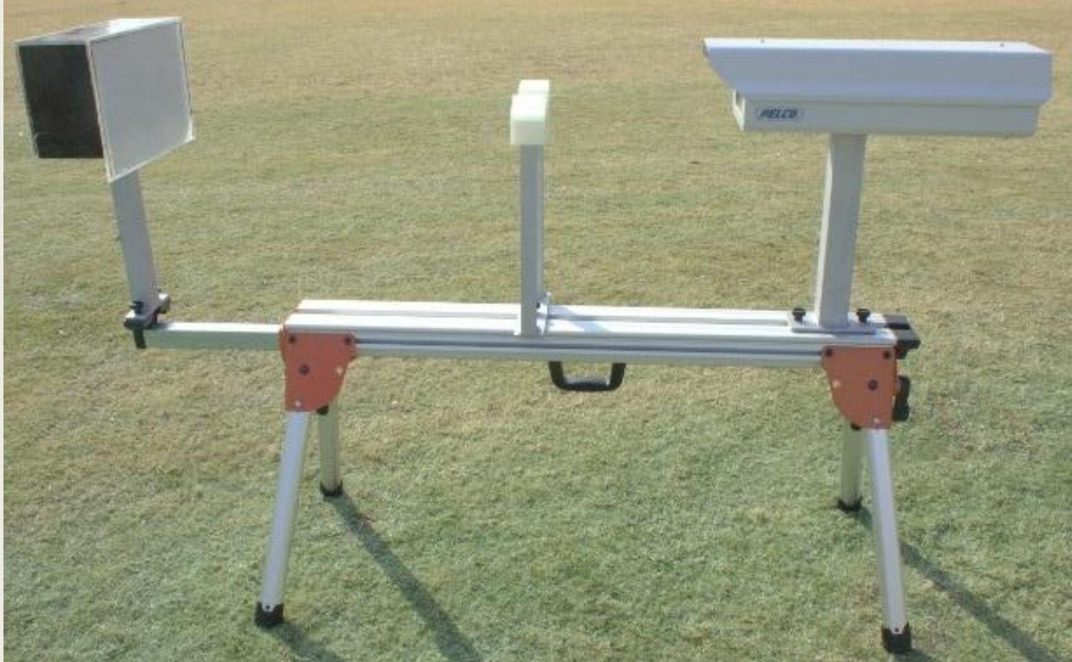
HOD system and main components: LED light (left), the sensor unit (middle), and the high-speed camera (right).
