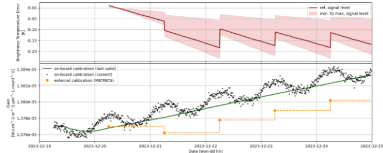
IR12.3 on-board vs. external gain calibration (stray light correction: on)
